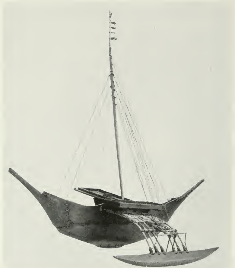
FIG. 30. Old canoe model. Present-day canoes lack the projections at the ends of the canoe, but otherwise details of construction are much the same. Model collected about 1900 (Cat. No. 91421-1).
