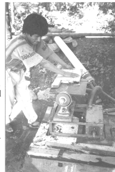
Watermotor Turbine powers Woodworking Tools www.watermotor.net , www.homepower.com
