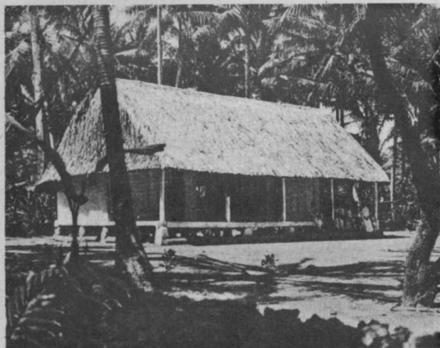
House of the High Chief of Ngatik. Major chiefs and the nobility were permitted to have houses of four sections (a section being the distance between the outer house posts, 6 feet, in terms of which the roof and walls were constructed). Commoners and lesser nobility had only two or three sections.
