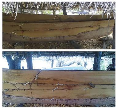
Figure 2: Asymmetrical stitching of canoe (Rico Roldan, 2016)
