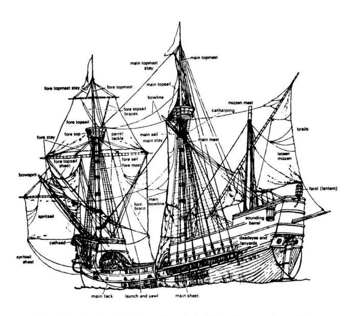
Magellan's flagship Trinidad may have looked like this. According to the best estimate, her dimensions were 25 meters in length, 7 meters in breadth, and 3 meters in depth of hold. (From W. D. Brownlee's First ships Around the World, Minneapolis, 1977)
