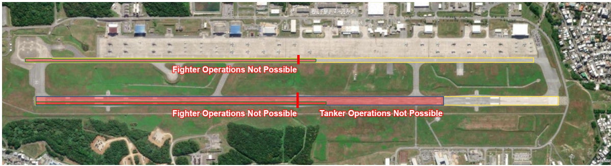
FIGURE 7. Open v. Closed Runway Crater Cuts – Denying All Aircraft Operations
