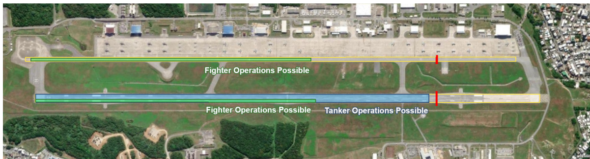
FIGURE 5. Open v. Closed Runway Crater Cuts – Insufficient Cuts
